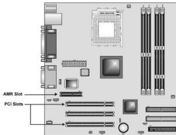
**PCI Slots** PCI slots are used to install expansion cards that have the 32-bit PCI interface.
