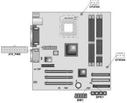
A top-down diagram of a mainboard with several connectors highlighted. On the left side, the ATX_PWR connector is shown. At the top, the CPUFAN connector is labeled. On the right side, the SYSFAN connector is labeled. At the bottom center, the SW1 header is labeled. At the bottom right, the SPK1 header is labeled. |
